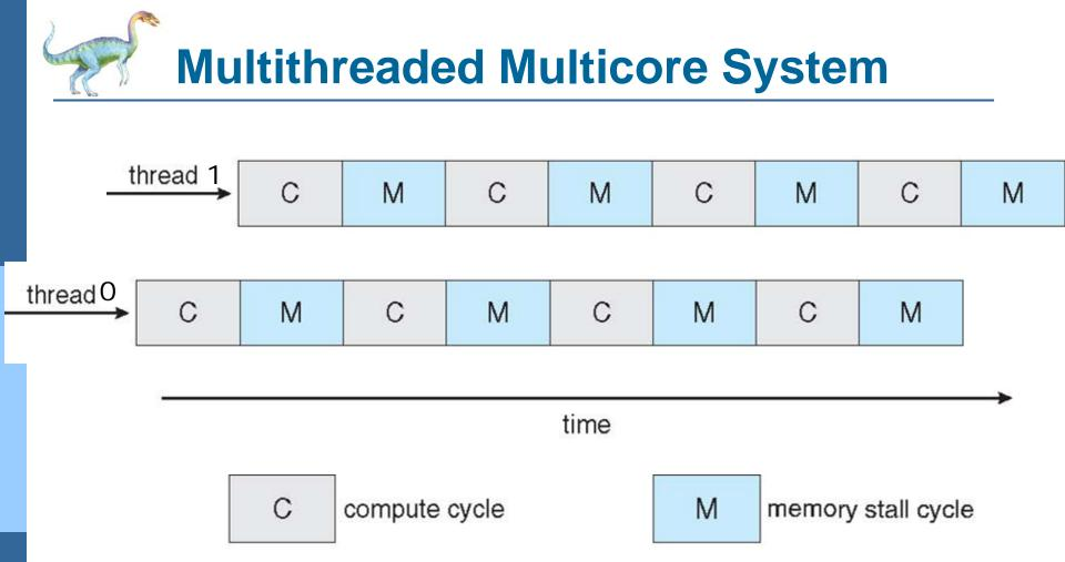
Multithreaded processor cores in which 2 (or more) heardware threads are assigned to each core.
