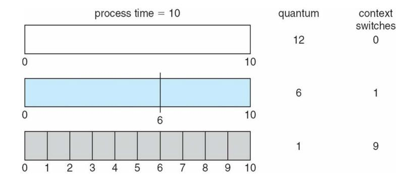
Showing how a smaller time quantum increases context switches
