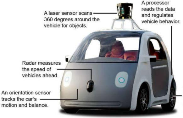
A wheel-hub sensor detects the number of rotations to help determine the car's location.
